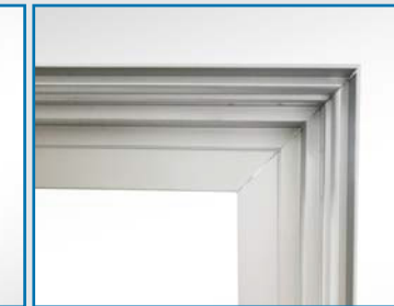
3. Check Angle for 90 degrees
